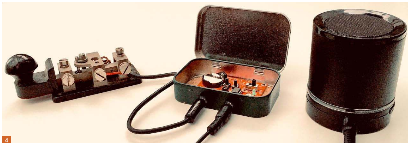
Fig. 4: The Morse tutor in a mint tin, with key and amplified speaker.
